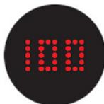
When connected to the ZEB Horizon RT that is powered on, two presses of the battery's display button will show a predicted run-time against the given load, expressed in hours and minutes.
