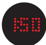
The Capacity display senses the orientation of the battery and adjusts to ensure legibility.
